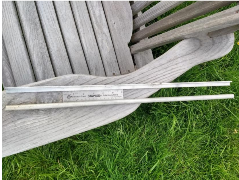
Photo 1 Example of Aluminum plot stakes for use as Reference Pins and IPC Pins
